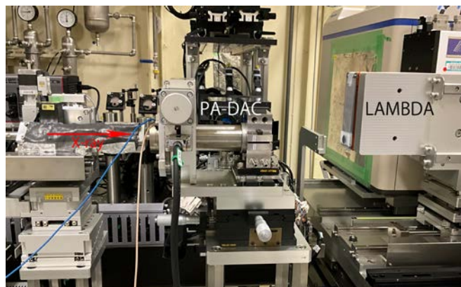
Fig.1. A prototype of PA-DAC system installed at SPring-8 (BL10XU).
