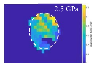
Fig.2. Magnetic flux density (MFD) image of the same region as Fig.1. The strength of MFD corresponds to the color bar. The image can not clearly define the sample shape.
